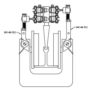
Torsion collectors mounted on a monorail Hoist/Trollev unit. The collector for the third conductor (TC1) will mount on the rear trolley hub, left side.
