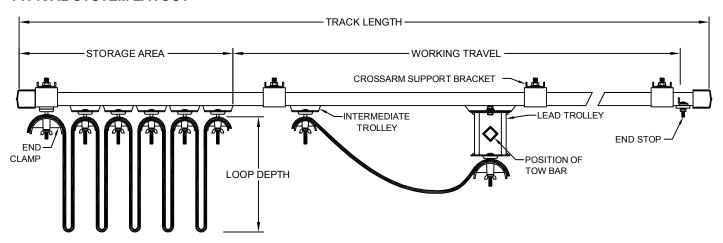
Use tow chains or straps for curved or high speed systems.
