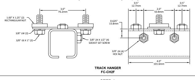
Install track hangers on crossarms, leaving clamping bolts loose.
