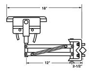
HD-300-PC Pantograph Collector, Single Shoe
