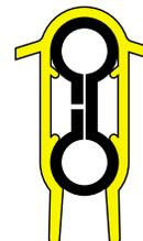
Cross-sectional drawing of Basic Figure 8 (FE) Conductor Assembly
