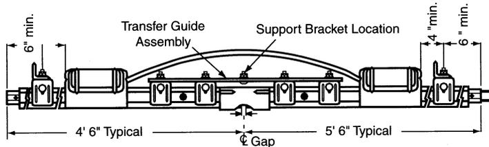
**The maximum gap opening for all ten foot Figure 8 expansion gap assemblies is 1-3/4 inches.**
